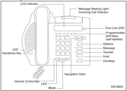
The M3903 has two Programmable Line (DN)/Feature Keys (self-labeled) with two features or lines (DNs) configured on each key. The M3903 also has four Context Sensitive Soft Keys (self-labeled).
