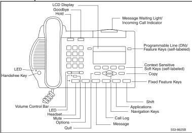
The **M3904** has six Programmable Line (DN)/Feature Keys (self-labeled), with two features or lines (DNs) configured on each key. The **M3904** also has four Context Sensitive Soft Keys (self-labeled).
